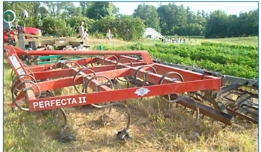
S-tine cultivator with sweeps, and a wheel that acts as a harrow on the back. Photo: Andy Pressman, NCAT
