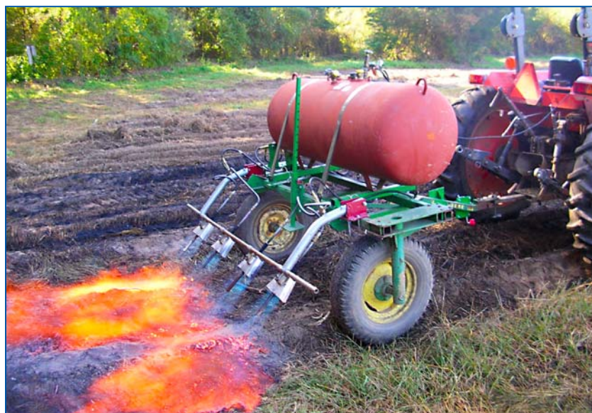
A tractor-mounted flame weeder in operation at Holcomb Farm in Connecticut. Smaller-scale flame weeders are also available, from hand-pushed weeders that span beds all the way down to backpack-mounted weeders. Photo: Courtesy of Holcomb Farm CSA
