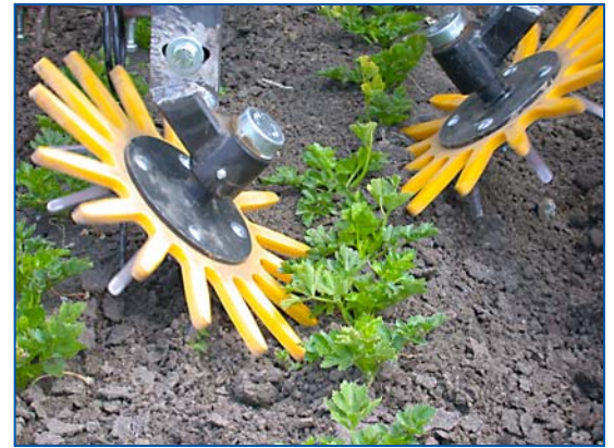
Finger weeders at work in celery transplants. Photo: Richard Smith, courtesy of UC Cooperative Extension
