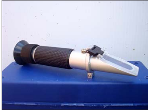
A refractometer can be used by growers to help manage crop health. Photo: Andy Pressman, NCAT
