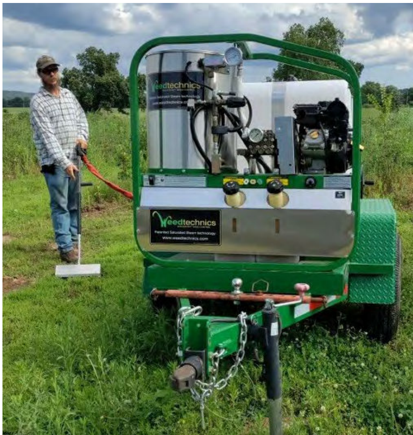
A steam-weeding device at the Arkansas blueberry farm of Megan and Matt (pictured) Varoz. Photo: Guy Ames, NCAT
