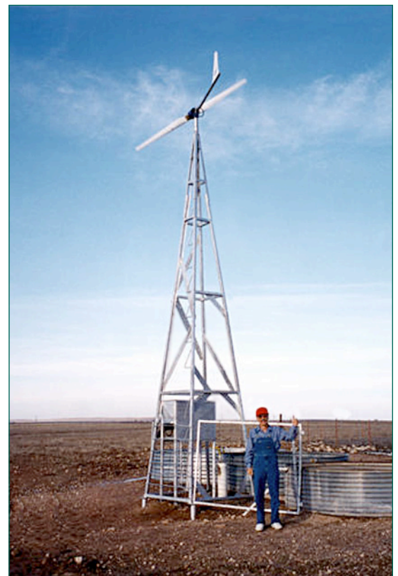
This 1-kW wind turbine from World Power Technology, Inc. is used for pumping water for 120 head of cattle at a ranch in Texas. Photo: World Power Technology
