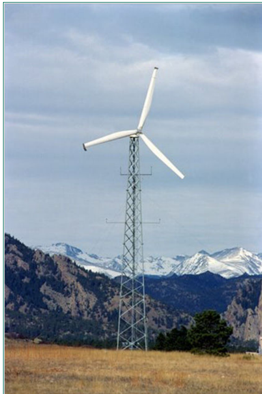
Horizontal-axis downwind machine. Photo: NREL, www.nrel.gov/data/pix/Jpegs/07301.jpg
