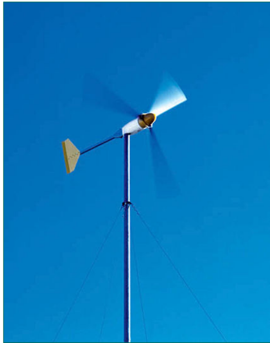
Caption: Bergey XL-1 horizontal-axis upwind machine. Photo: NREL, www.nrel.gov/data/pix/Jpegs/11238.jpg
