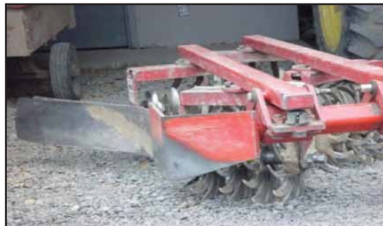
Figure 7: This Lilliston cultivator can be used for light tillage for weed control in the top few inches of soil as well as for incorporation of cover crop residues.
