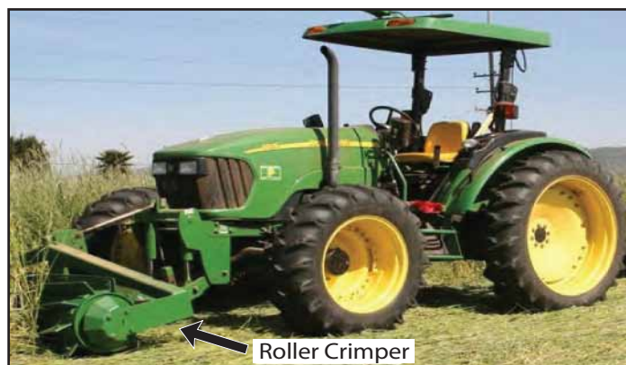
Figure 16: This rye cover crop was terminated using a roller crimper. (Eric Brennan)
