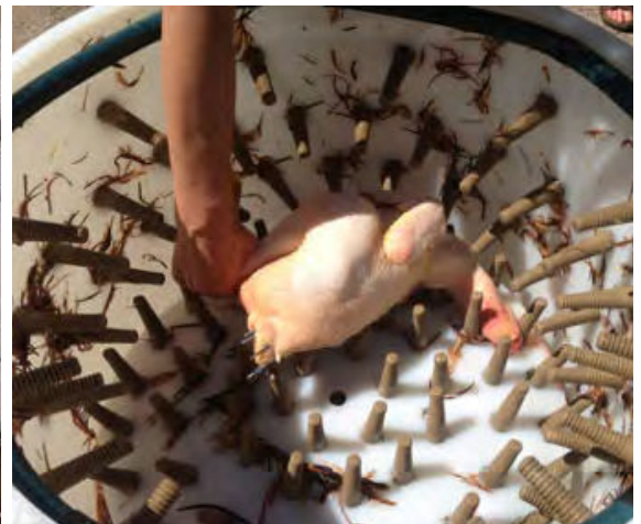
Appropriate equipment, such as this small-scale plucker, facilitate on-farm processing. Photo: Ann Baier, NCAT
