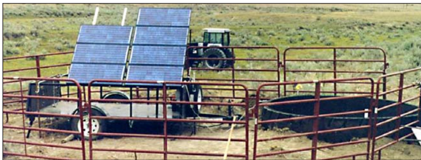
A trailer-mounted PV system is improving range management and water quality along Painted Robe Creek near Lavina, Montana. Photo: NCAT
