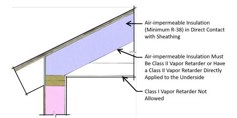
Unvented Attic: Air-impermeable Insulation Only (IRC R806.5)
