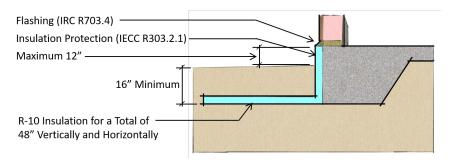
Insulation materials used below grade must be labeled as complying with ASTM C578. The discussion here addresses stand-alone structures. The IRC includes more details and specific requirements when a FPSF is adjacent to a heated structure and when a FPSF is adjacent to an unheated slab-on-grade structure. Refer to IRC R403.
