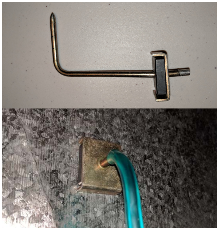
Figure 7-6. Static Pressure Probe Pressure probe may be inserted into the trunk duct pointed toward the air handler fan.
