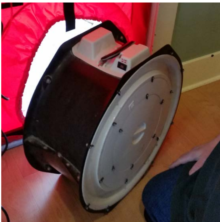
Figure 6-14. Mounting Blower Door Fan in Frame
