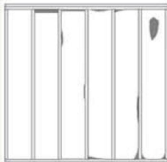
Compression or incomplete fill: <2% of area, compressed by <30% of intended thickness
