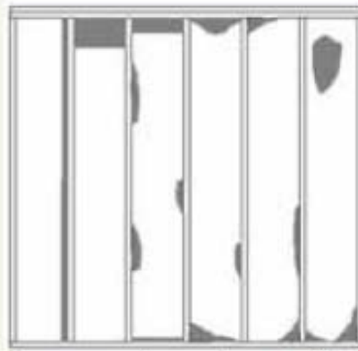
Compression or incomplete fill: <10% of area, compressed by <30% of intended thickness
