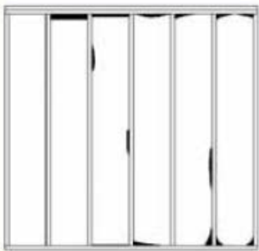
Gaps clear through insulation: <2%
