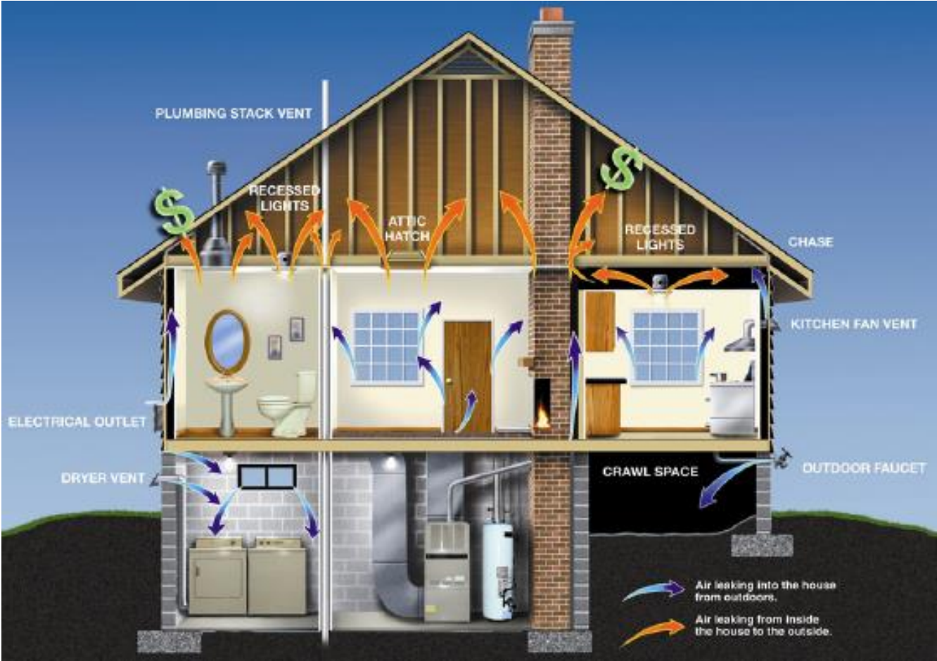
Unintentional Air Leaks (Source US EPA)
